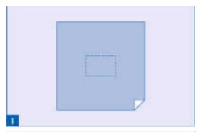
Place sterilization supplies (e.g. instrument tray) on centre of paper.
