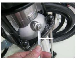
Figure 4-1: Open the bleeding screw
