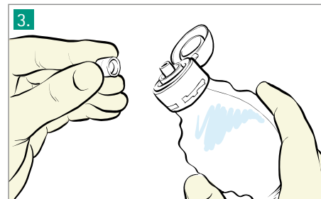
3. Twist off the closing cone from the filling port and place it on a sterile surface.
