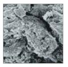
The roughened surface area provided by the osteoconductive Plasmapore<sup>xp®</sup> coating delivers enhanced implant stability.1
