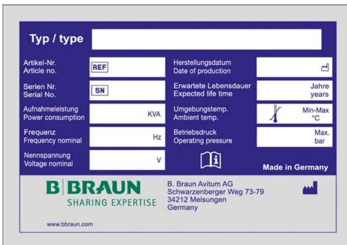
Figure 6-1: Example of a type plate
