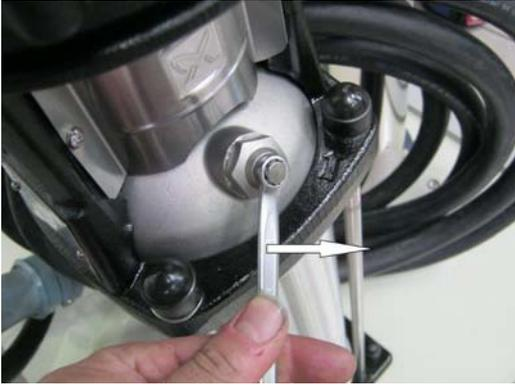
**Figure 4-1: Open the bleeding screw**
