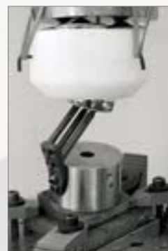
Set-up for biomechanical Targon® FN lab testing
