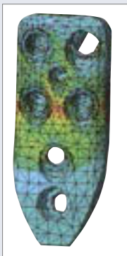
stress peaks in plate and sleeves
