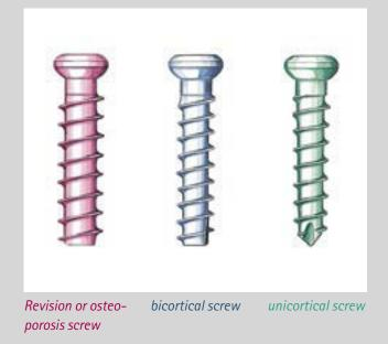
The selection of drill guides and drills depends on the screw fixation technique. If unicortical screws are to be used (colour coded green) the FG414R drill (diameter 2.2 mm) should be used, with the corresponding double drill guide FG415R (green handle).
